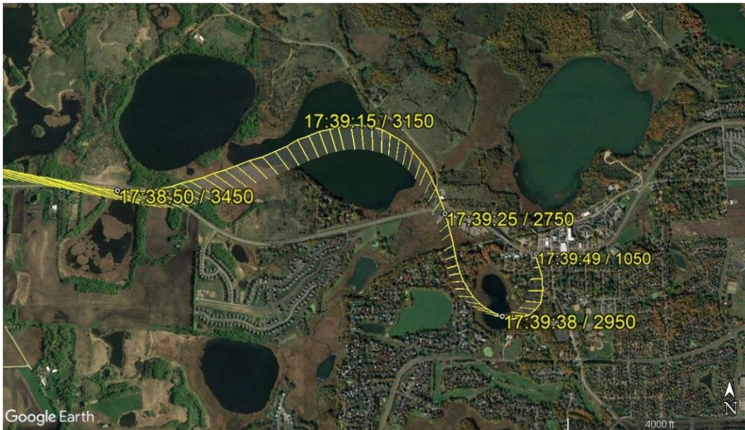
**Figure 3.** Flightpath showing increasingly tight turns with times and altitudes (in msl).
